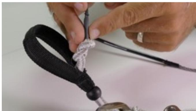
12. Pull this knot tight while still making sure that the end of the mark cloth is still visible.
