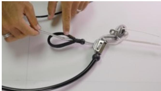
11. Tie a figure of 8 knot on the line making sure that the end of the Mark Cloth is visible after the knot.
