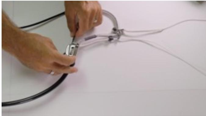
10. Pass the end of the trim line through the new Trim Handle that was supplied, and pull the line through so that the bungee connection is below the handle.
